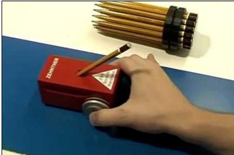
**Interpretir** *This simple metal "car" produces more consistent test results by providing consistency in the angle and pressure during the Pencil Hardness test procedure* scratch the surface is the reported surface harness level.
