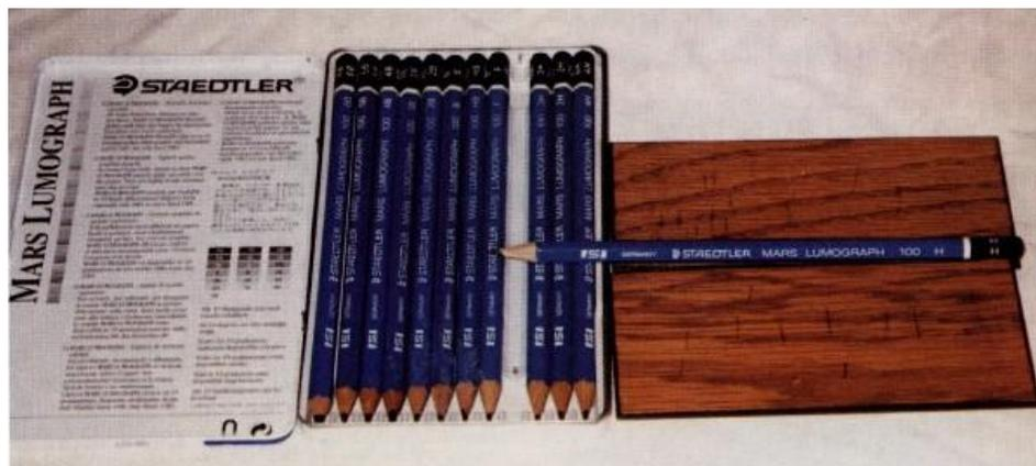
*A set of calibrated test pencils intended for measuring Pencil Hardness*
