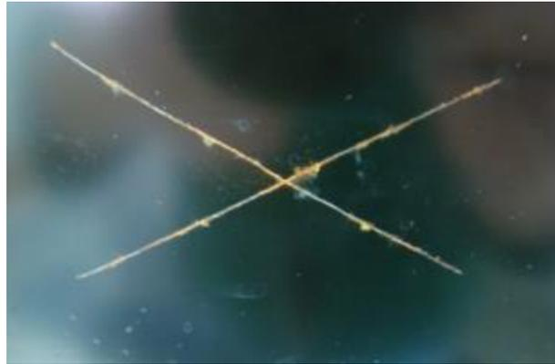
Pencil hardness is a measure of how resistant a coating film is to fracture due to friction from a sharp object. The underlying idea of the test is that an object made of a hard material will scratch an object made of a softer material. When testing coatings, measuring scratch hardness can be accomplished in two related ways.
