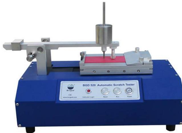
*This device uses varying pressure, and measures the force required to scratch the surface.*
